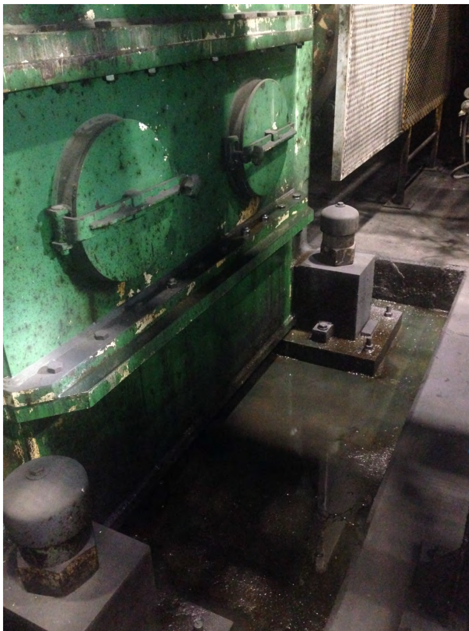
Oil pooling around the base of the unit
