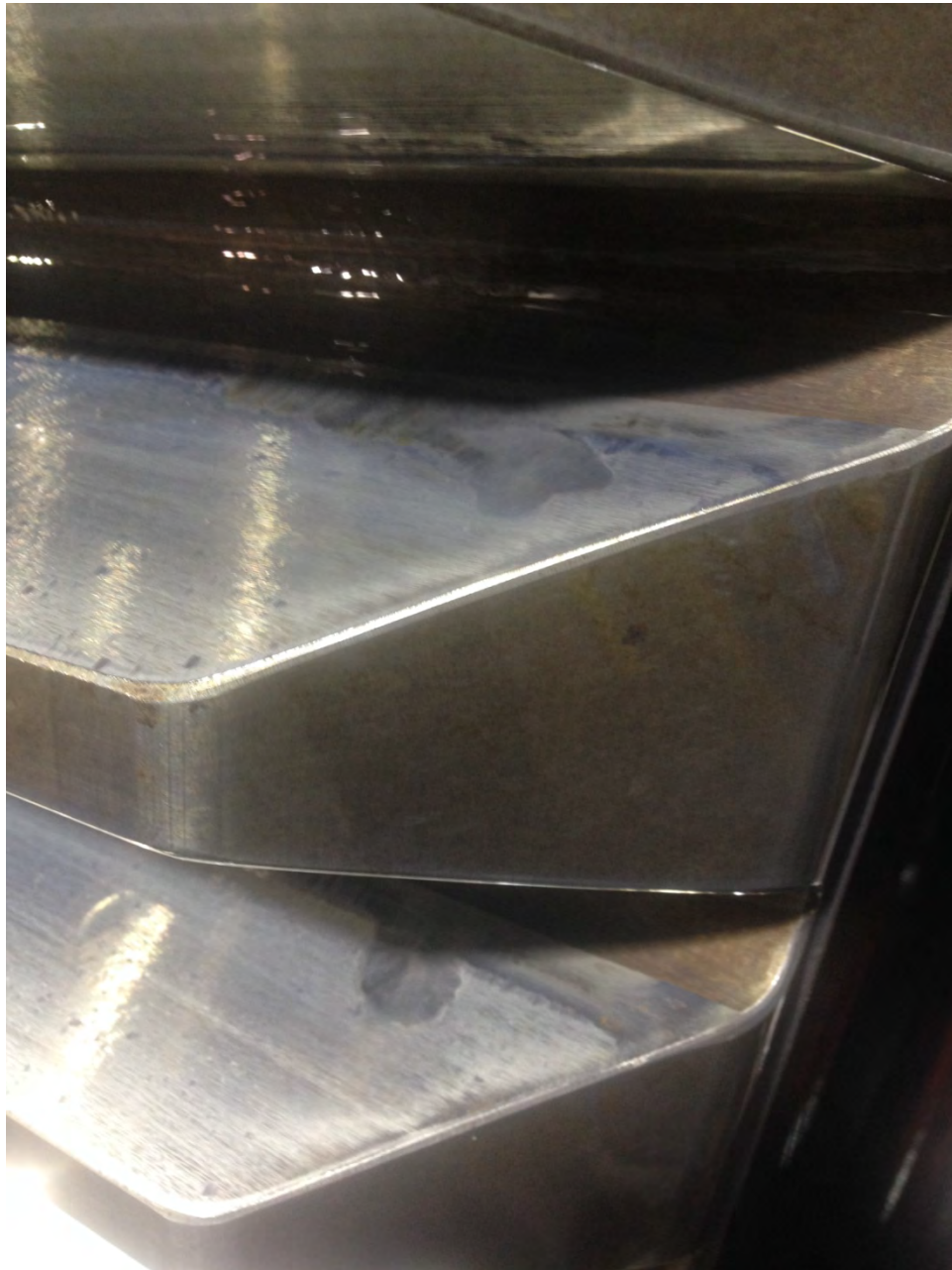
Close-up of the Gear Tooth blemishes on Main Drive 1
