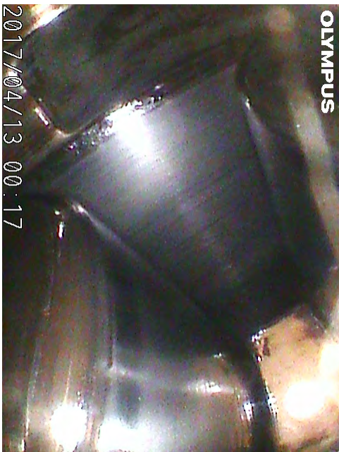
F2 Bottom Motor Bearings showing rust
